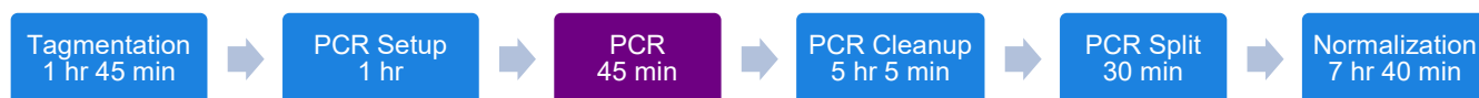
Figure 1. Workflow overview for NGS library preparation on the Apollo system with the Nextera XT library prep kit. Blue and purple boxes indicate steps performed on and off the Apollo system, respectively. Indicated times are estimates for completion of each protocol, and include reagent and equipment setup, heating/cooling/thawing of reagents and hardware, incubation of reactions, and automated liquid-handling processes.
