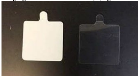
Figure 14. Sealing film and imaging film. The sealing film (left) is provided with a white backing. The imaging film (right) is double sided and is provided between two layers of clear backing.
