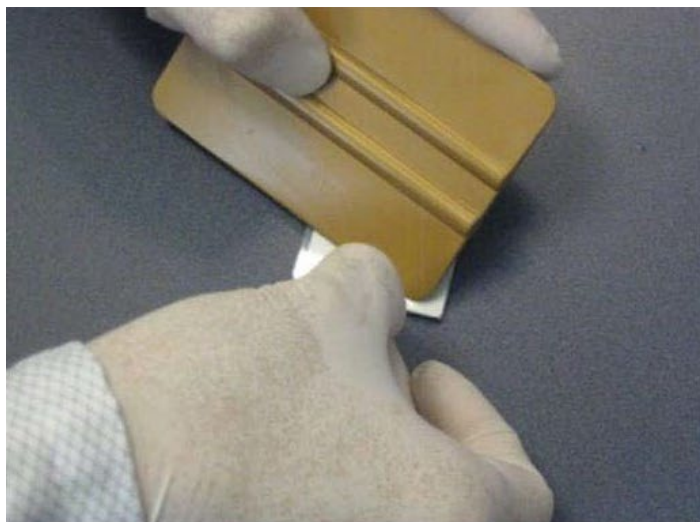
Figure 15. Sealing the blotted chip. Seal the blotted chip using a Film Applicator (left). The tab of the imaging film should be oriented downward relative to the chamfered corner of the chip (right).
