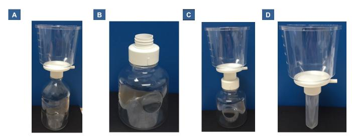
Figure 1. Setting up the Capturem His-Tagged Purification Large Volume Unit. The Capturem His-Tagged Purification Large Volume Unit connects directly to a 33-mm diameter thread bottle (Panel A). The provided Bottle Thread Adaptor (Panel B) allows the purification unit to connect to a 45-mm diameter thread bottle (Panel C). The purification unit connects directly to a 50-ml tube for elution (Panel D).
