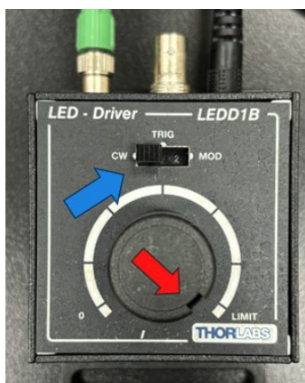
Figure 12. Required settings on the UV meter (1.2 A).
