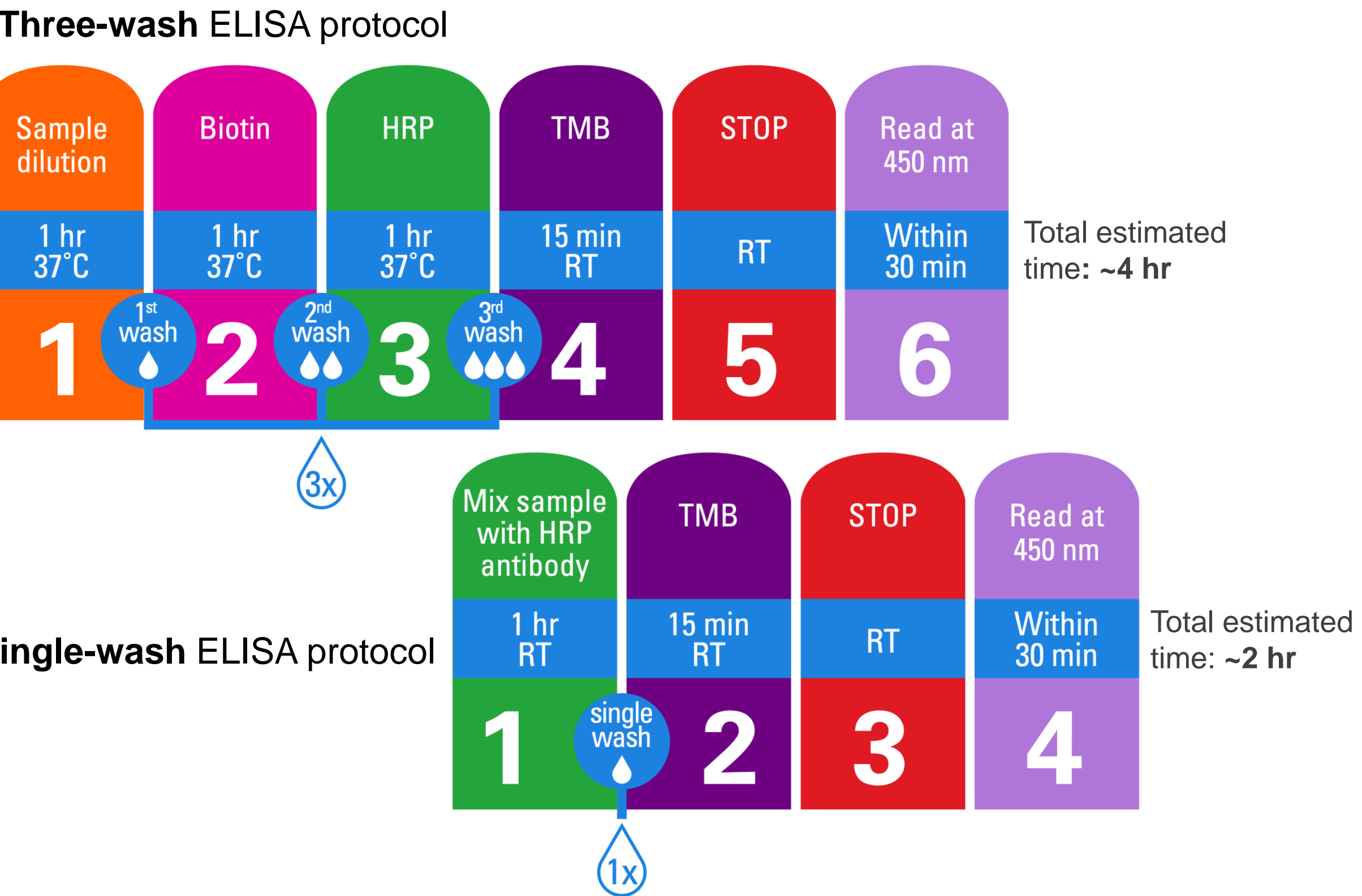
Figure 2. AAV Rapid Titer ELISA Kit (Single Wash) protocol involves fewer overall steps, including only a single wash step. This protocol simplifies the process and reduces hands-on time and effort for titer determination.
