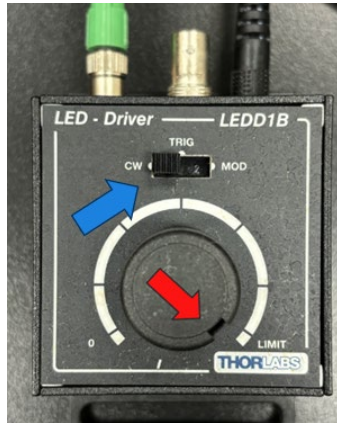
Figure 12. Required settings on the UV meter (1.2 A).
