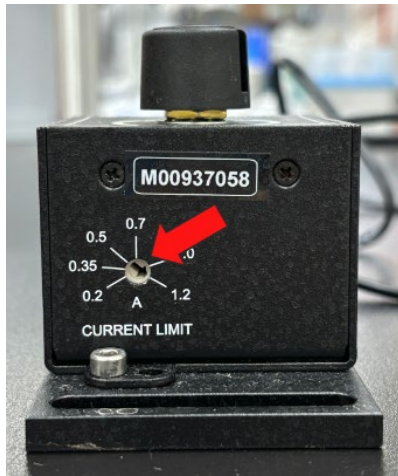
Figure 6. Correct setting shown on the UV meter (1.2 A).
