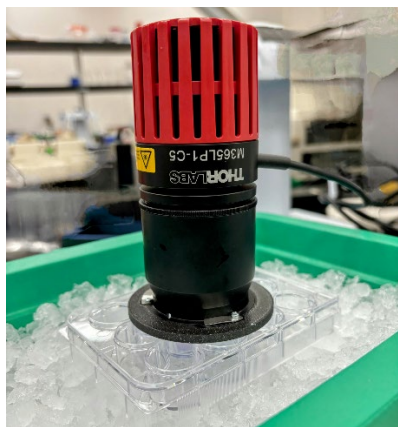
Figure 11. Placement of the UV lamp on the well and tile.
