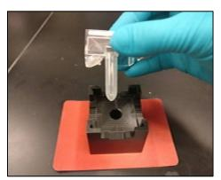
Figure 77. Removing the Collection Tube containing the eluate.
