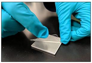
Figure 74. Removing the film from the chip.
