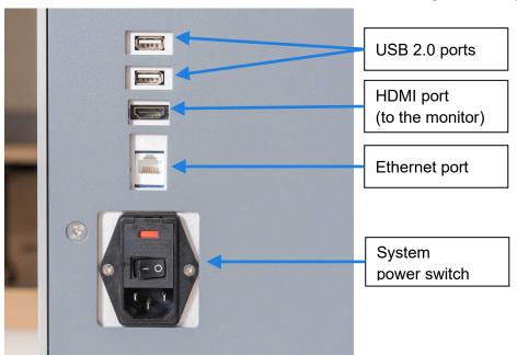
Figure 3. Identification of the electrical input and output on the back of the Shasta Single Cell.
