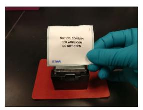
Figure 76. Securing the collection module with Collection Film.
