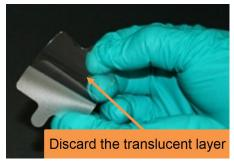
**Figure 66. Preparing and adhering RC Film.** RC Film is composed of two layers: one clear and the other translucent. When sealing a chip, remove the translucent layer and discard it. Put the remaining layer on the chip.
