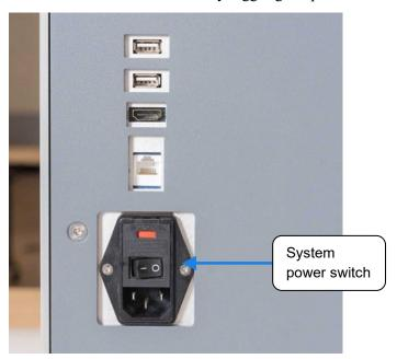
Figure 84. Location of the system power switch.
