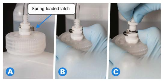
Figure 79. Visual aid for how to remove the tubing connector from the water source bottle, humidifier source bottle, and the waste container.
