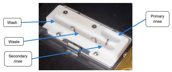
Figure 11. Tip wash trough well locations.
