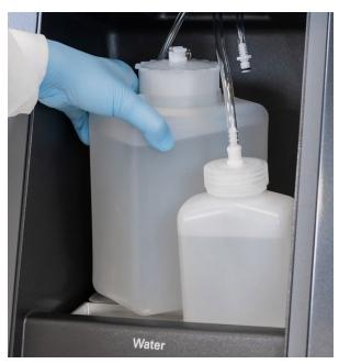
Figure 80. Removing the water bottle from the Shasta instrument.
