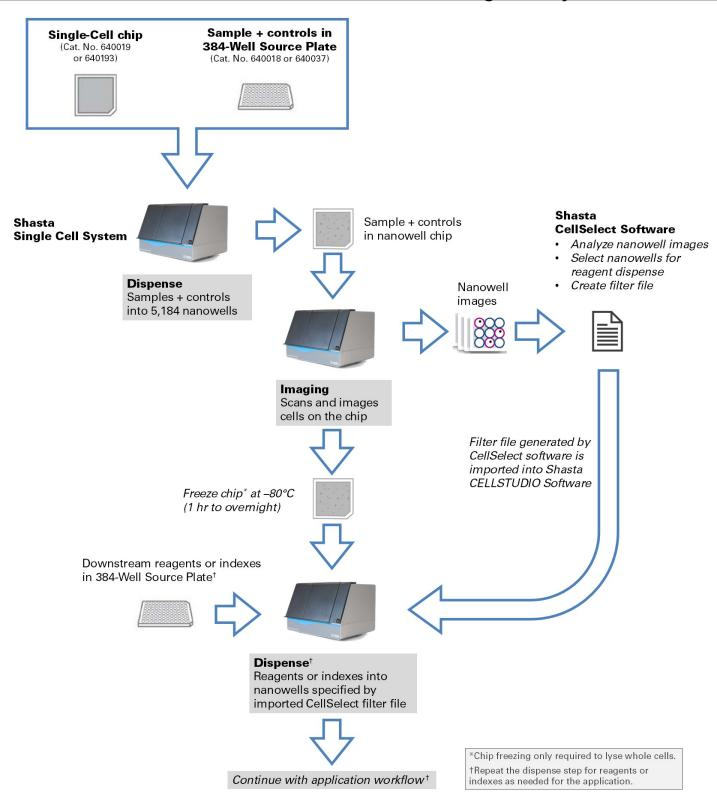
Figure 15. Shasta dispense and cell scan workflow.
