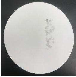
Figure 64. Examples of blotting results. (Left) Example of an acceptable result; the red marks indicate spots on the paper where blots were observed prior to evaporation. (Right) Example of a poor blot; note the size and quantity of the damp spots on the paper.
