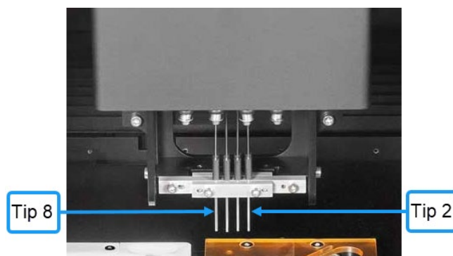
Figure 63. Tip numbering identification visual guide. When looking into the Shasta instrument from the open door, Tips 2, 4, 6, and 8 are the ones visible (in the front, right to left) of the tip nozzle assembly. See Table 5 for the top-down map.
