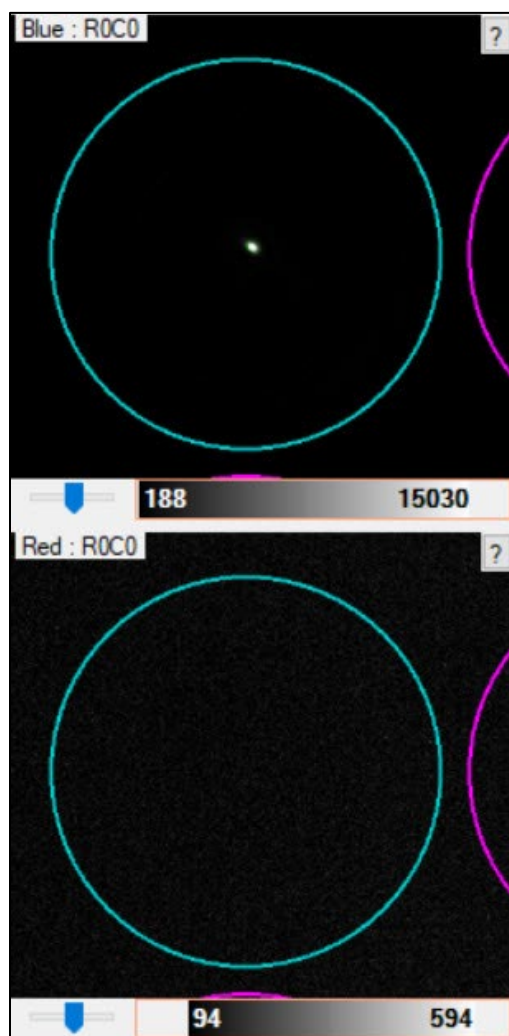
Figure 55. Single-well image from a two-color chip scan of cells stained with Hoechst (Blue channel) and propidium iodide (Red channel). The top image shows a signal (cells that have absorbed Hoechst dye), which indicates the presence of a live cell; the bottom image would show a signal from propidium iodine staining (if present). In this example, the well matches the designated candidate logic selection parameters (see Section II.C.1) and is, therefore, a candidate. If objects appear in the bottom image only or both the top and bottom images, they are either dead cells, other debris, or an imaging artifact.
