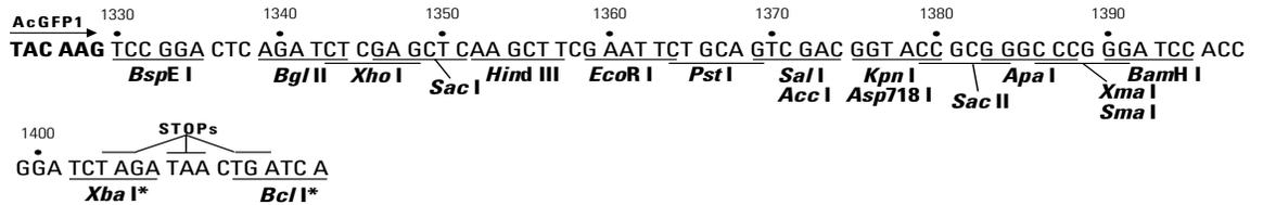
**Restriction Map and Multiple Cloning Site (MCS) of pAcGFP1-C1.** Restriction sites shown in bold are unique. The *Xba* I and *Bcl* I sites (\*) are methylated in the DNA provided by Clontech Laboratories, Inc. . If you wish to digest the vector with these enzymes, you will need to transform the vector into a *dam*<sup>-</sup> host and make fresh DNA.
