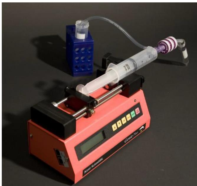
**Figure 3. Placement of the Adeno-X Purification Assembly on an infusion pump.** A pump from Kent Scientific is shown, but any infusion syringe pump will work.
