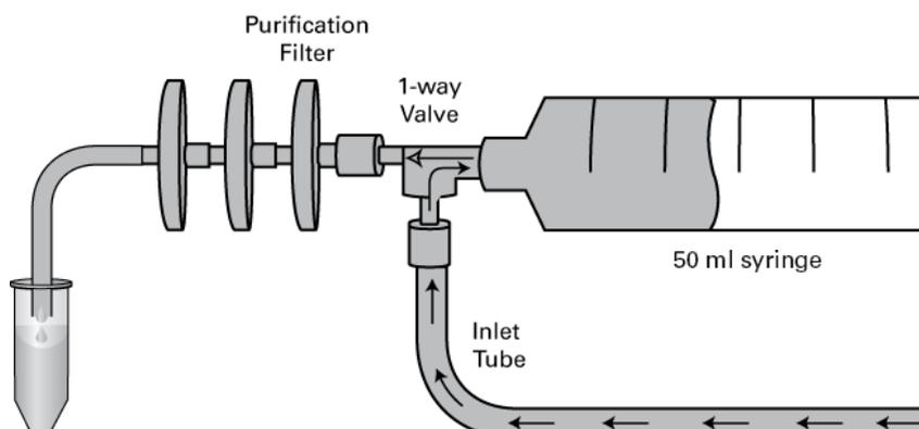
**Figure 1. The Adeno-X Mega Purification Assembly.** The apparatus comes pre-assembled.
