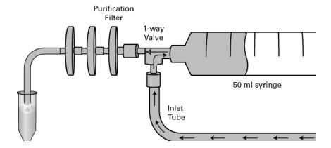
Figure 1. The Adeno-X Mega Purification Assembly. The apparatus comes pre-assembled.
