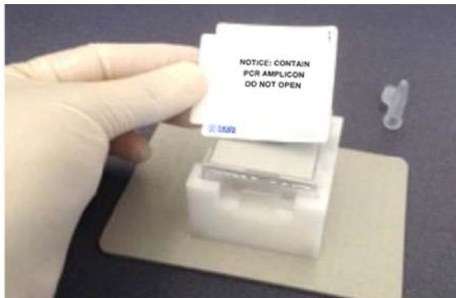
Figure 48. Securing the collection module with Collection Film.
