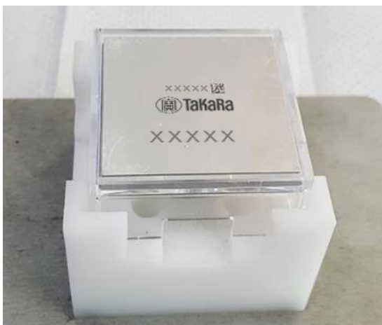
Figure 47. Placing the chip into the collection module.
