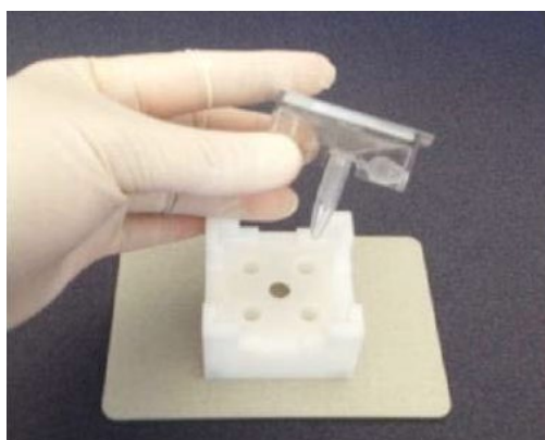
Figure 49. Removing the Collection Tube containing the eluate.
