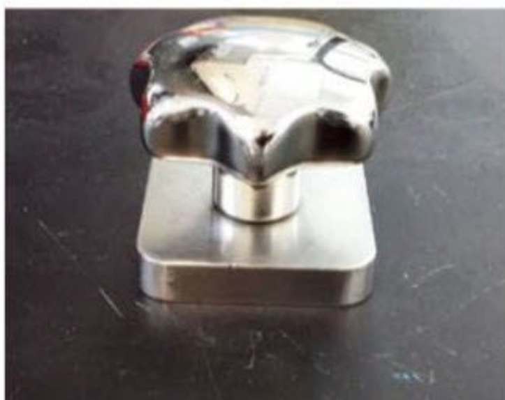
Figure 11. Blot the chip with Blotting Paper and Blotter. A Blotter is provided with the ICELL8 Single-Cell System.
