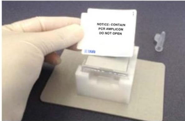
**Figure 43. Securing the Collection Module with Collection Film.**
