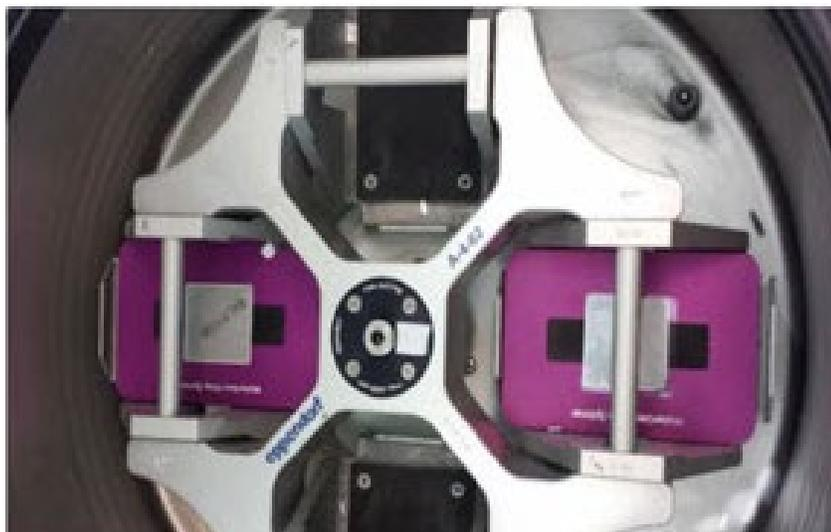
Figure 15. Centrifuge Chip Spinner.
