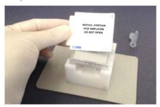
Figure 43. Securing the Collection Module with Collection Film.
