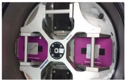
Figure 15. Centrifuge Chip Spinner.
