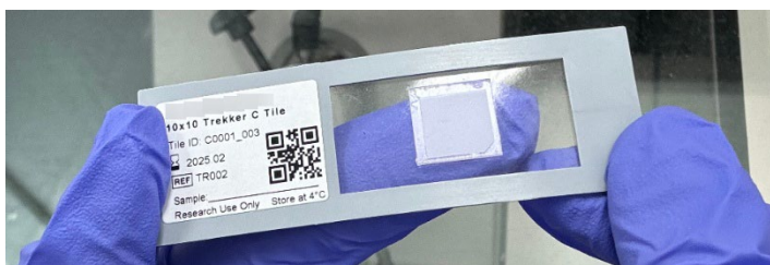
Figure 10. Demonstration of the precise placement method onto the tissue region of interest.
