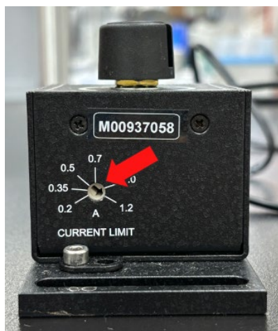
Figure 6. Correct setting shown on the UV meter (1.2 A).
