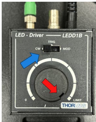
Figure 12. Required settings on the UV meter (1.2 A).
