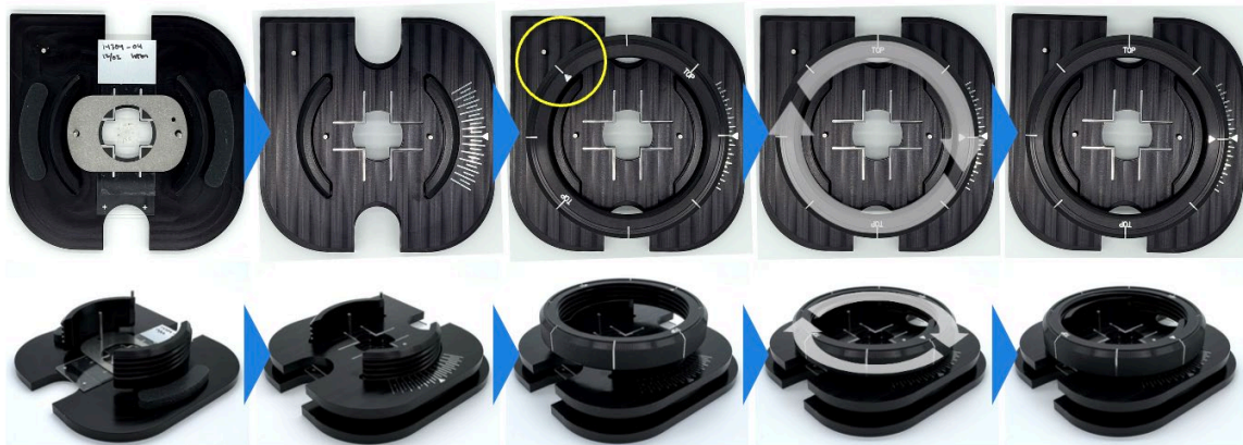
Figure 9. Step-by-step assembly of the Trekker Alignment Fixture. Align the asymmetric corners of the Top and Bottom plates, then combine the plates with the Tile and Tissue slide facing each other. Install the Tightening ring, with the arrow pointing toward the top-left guide pin to engage the threads and turn clockwise to sandwich the two slides.
