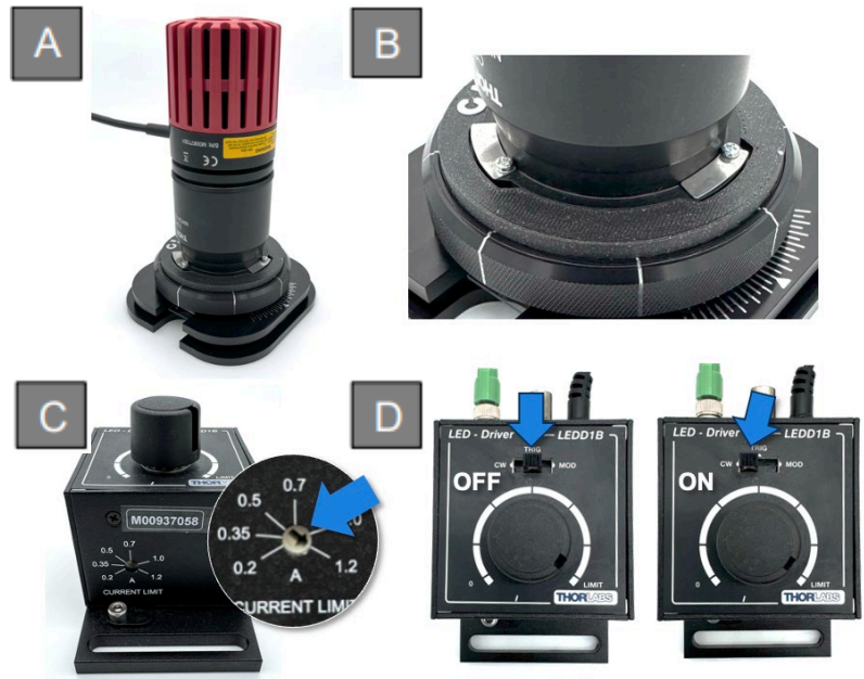
Figure 16. UV lamp for the Trekker Alignment Fixture. Panel A. Diagram depicting the placement of the UV lamp on the assembled Trekker Alignment Fixture. Panel B. The UV lamp should fit securely within the bevel of the fixture’s Tightening Ring. Panel C. Prior to operation, the UV meter should be set at 1.2 A. Panel D. The UV lamp is turned on by flipping the switch to the left to (CW).
