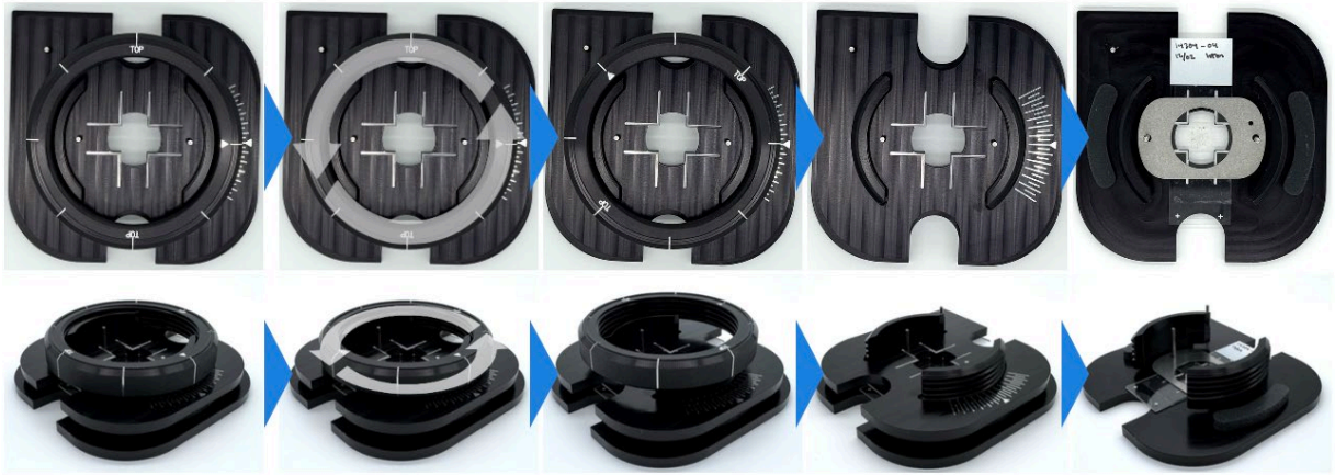
Figure 11. Step-by-step disassembly of the Trekker Alignment Fixture. Gently rotate the Rightening Ring counterclockwise to slowly separate the Top and Bottom plates. Carefully remove the Tightening Ring and the Top Plate without touching the tissue. Remove the Tissue slide from the Bottom Plate and proceed to the next steps of the protocol.
