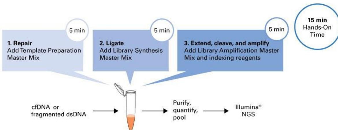
**Figure 1. ThruPLEX Tag-Seq HV single-tube library preparation workflow.** The ThruPLEX Tag-Seq HV workflow consists of three simple steps that take place in the same PCR tube or well and eliminates the need to purify or transfer the sample material.
