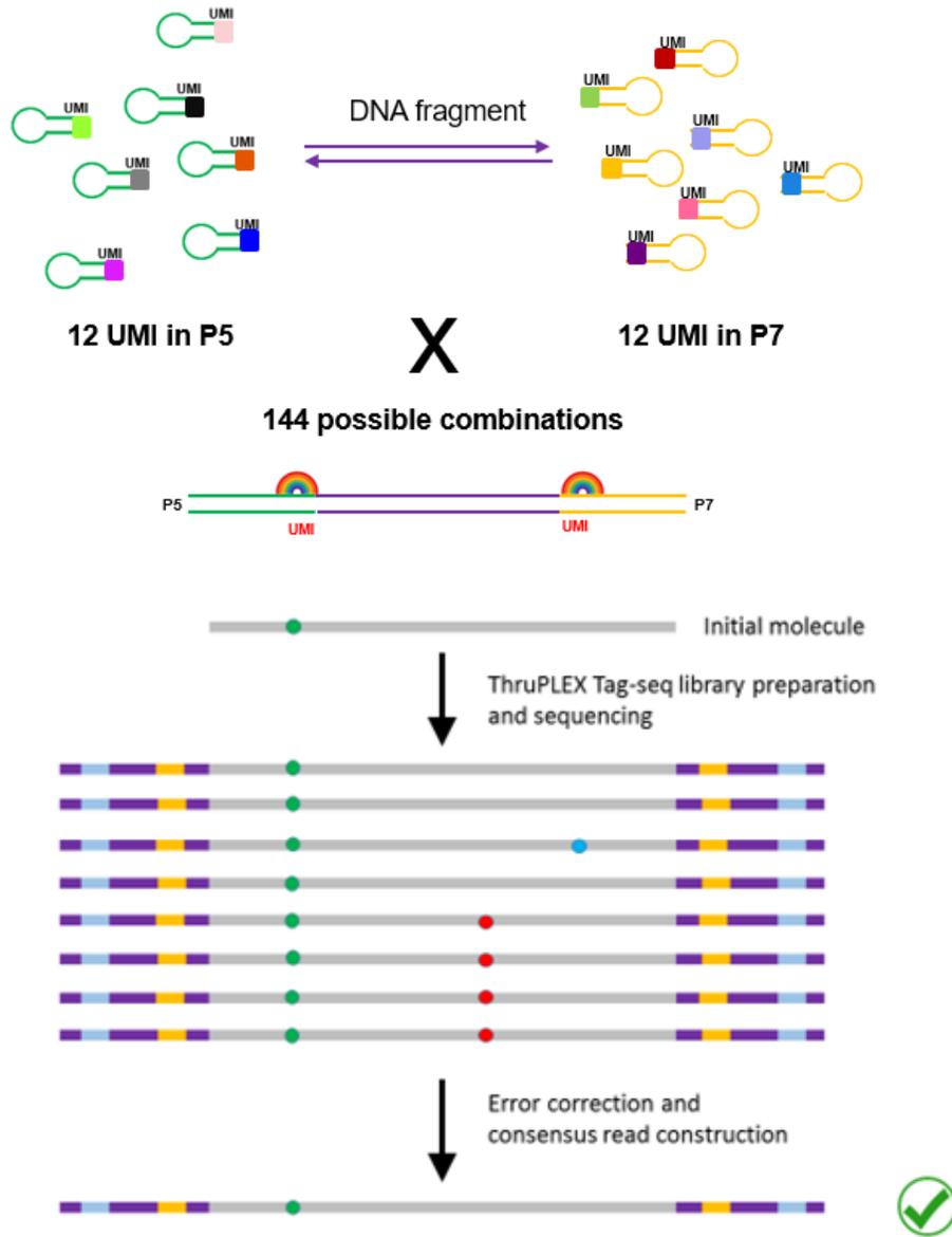
**Figure 3. ThruPLEX Tag-Seq HV contains 144 discrete unique molecular identifiers (UMIs).** The ThruPLEX Tag-Seq HV is designed to remove the ambiguity in variant calling by reducing the false positive calls coming from DNA polymerase and sequencing errors. The seven base UMIs are located at the beginning of the reads ensuring an easy demultiplexing of the samples to simplify the analysis
