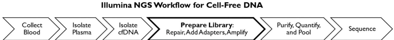
**Figure 1. Illumina NGS workflow for cfDNA** Blood samples are collected, plasma is isolated, and cfDNA purified. ThruPLEX Plasma-seq library preparation follows and consists of three steps: repair, ligation and amplification. Indexed libraries are purified, quantified, and pooled prior to sequencing on Illumina NGS platforms.
