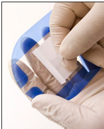
Figure 42. Removing the backing from the Cycler Sealing and Pressure Film.
