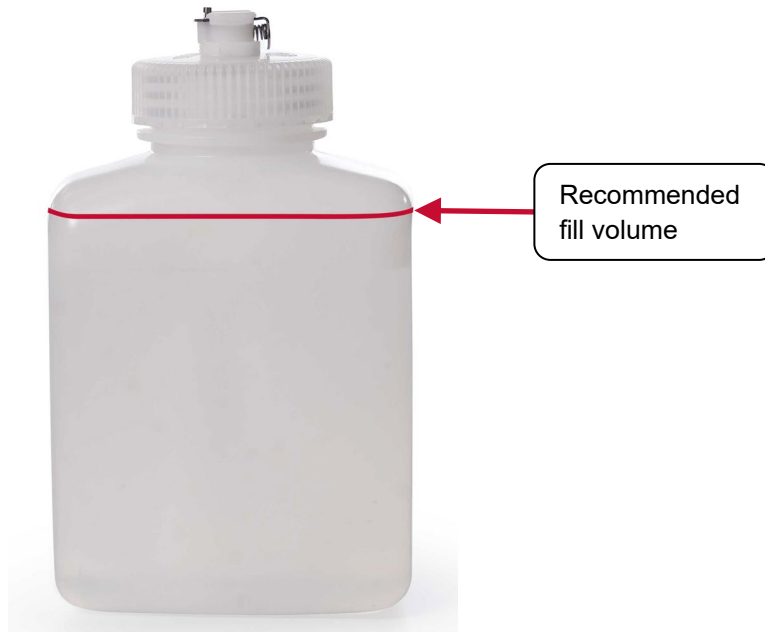
Figure 48. Visualization of the recommended fill volume of the humidifier source bottle. The water level should be below where the bottle begins to curve to the top.
