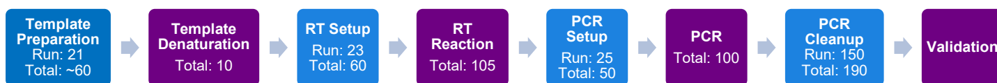
Figure 1. Workflow for cDNA preparation with the Apollo system and the SMART-Seq v4 Reagent Kit for the Apollo System. Blue and purple boxes indicate subprotocols performed on and off the Apollo system, respectively. Run = the run time in minutes on the Apollo system, if applicable. Total = total time in minutes spent, including thawing of reagents, reagent and equipment setup, heating and cooling of thermal blocks, incubation of reactions, and automated liquid-handling processes, if applicable. Run time is independent of sample number. Validation time varies depending on the method used.
