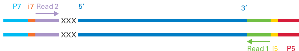
Figure 5. Structural features of final libraries generated with SMART-Seq® Total RNA Single Cell Library Prep with ZapR® Depletion. The adapters added during PCR 1 contain sequences allowing clustering on Illumina flow cells (P7 shown in light blue, P5 shown in red), indexes for pooling multiple samples in a single sequencing lane (Index 1 [i7] sequence shown in orange and associated with the P7 sequence, and Index 2 [i5] sequence shown in orange and associated with P5 sequence), as well as the regions recognized by sequencing primers Read Primer 2 (Read 2, purple) and Read Primer 1 (Read 1, green). Read 1 generates sequences antisense to the original RNA, while Read 2 yields sequences sense to the original RNA (orientation of original RNA denoted by 5' and 3' in dark blue). The first three nucleotides of the second sequencing read (Read 2) are derived from the SMART-Seq Stranded Adapter (shown as XXX). It is best to trim these three nucleotides prior to mapping if performing paired-end sequencing.
