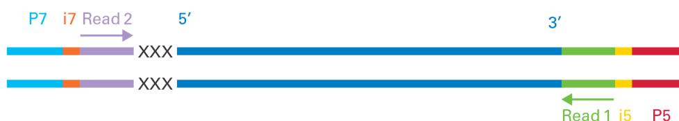
Figure 3. Structural features of final libraries generated with the SMART-Seq Stranded Kit. The adapters added during PCR1 contain sequences allowing clustering on Illumina flow cells (P7 shown in light blue, P5 shown in red), indexes for pooling multiple samples in a single sequencing lane (Index 1 [i7] sequence shown in orange and associated with the P7 sequence, and Index 2 [i5] sequence shown in orange and associated with P5 sequence), as well as the regions recognized by sequencing primers Read Primer 2 (Read 2, purple) and Read Primer 1 (Read 1, green). Read 1 generates sequences antisense to the original RNA, while Read 2 yields sequences sense to the original RNA (orientation of original RNA denoted by 5' and 3' in dark blue). The first three nucleotides of the second sequencing read (Read 2) are derived from the SMART-Seq Stranded Adapter (shown as Xs). It is best to trim these three nucleotides prior to mapping if performing paired-end sequencing.
