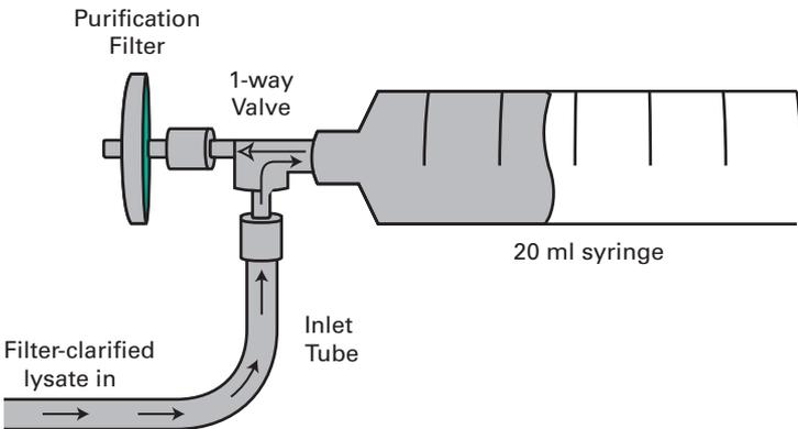
**Figure 2. The Adeno-X Maxi Purification Assembly.** The apparatus comes pre-assembled.
