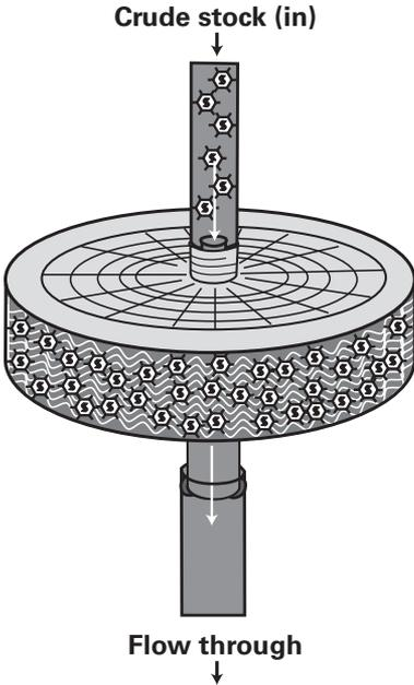
**Figure 1. Principle of Adeno-X virus purification.** The Adeno-X Purification Filter consists of several layers that selectively bind adenoviral particles as they pass through. The filter is enclosed in a small cylindrical cartridge that resembles a radial flow column, complete with entrance and exit ports. The Maxi purification cartridge is 3.5 cm wide and 1 cm thick.
