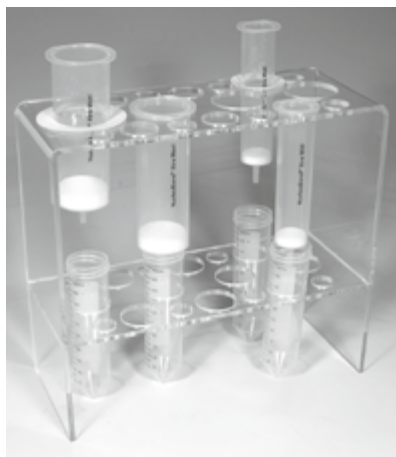
Figure 3 Setup of NucleoBond® Xtra Midi/Maxi Columns with the NucleoBond® Xtra Combi Rack
