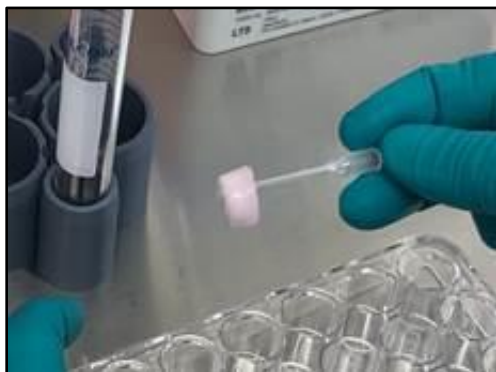
Figure 5. Transferring the sponge to a 15 ml tube using a 20 µl pipette tip.
