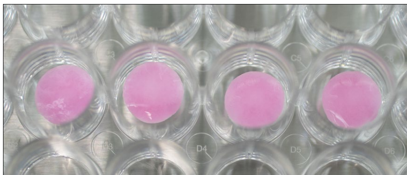
Figure 5. Proper placement of the sponge and sample in a well. The sponge is not touching walls, and the transduction mixture is all on the sponge.
