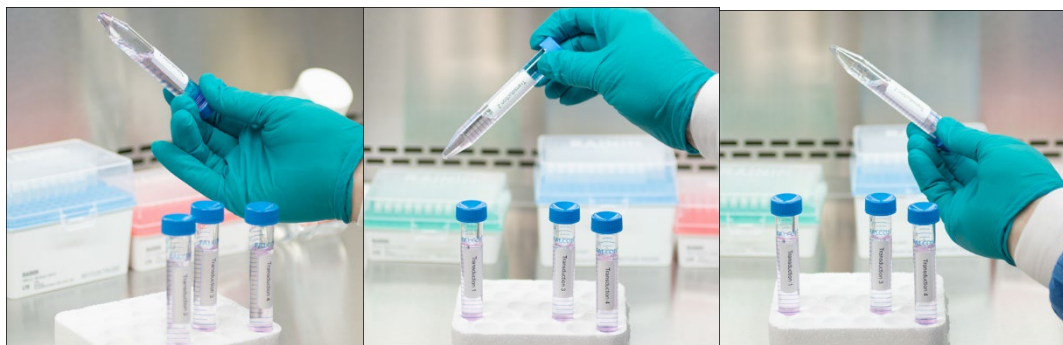
Figure 13. Gentle mixing by inversion. Invert and return upright a total of five times.
