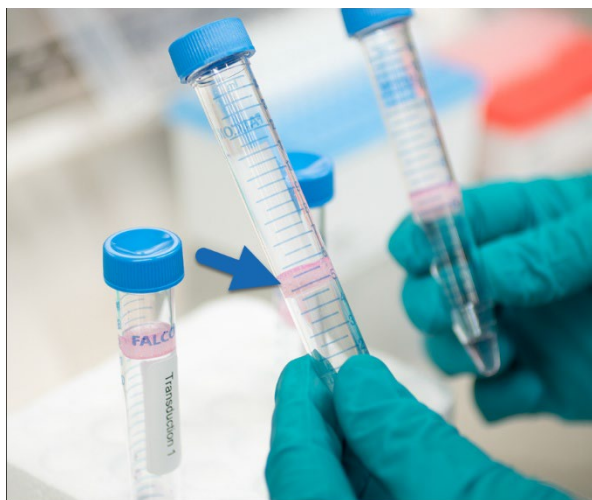
Figure 9. A 15 ml tube containing culture media, the sponge (arrow), and Release Buffer before centrifugation.
