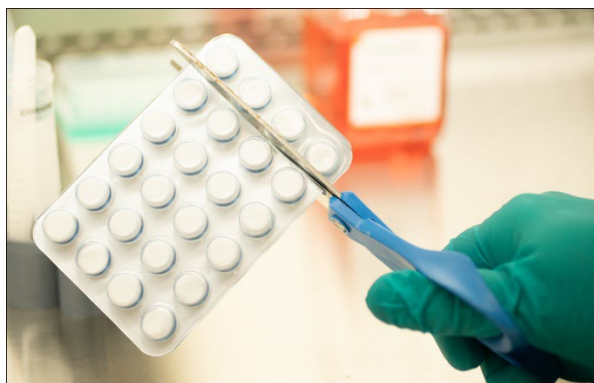
Figure 2. Proper cutting of the packaging to remove Lenti-X T-Cell Transduction Sponges. Cut between the wells of the blister package. Take care not to disturb the seal on adjacent wells.
