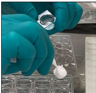
Figure 2. Transferring the sponge to a single well of a sterile, 24-well non-treated tissue culture plate.
