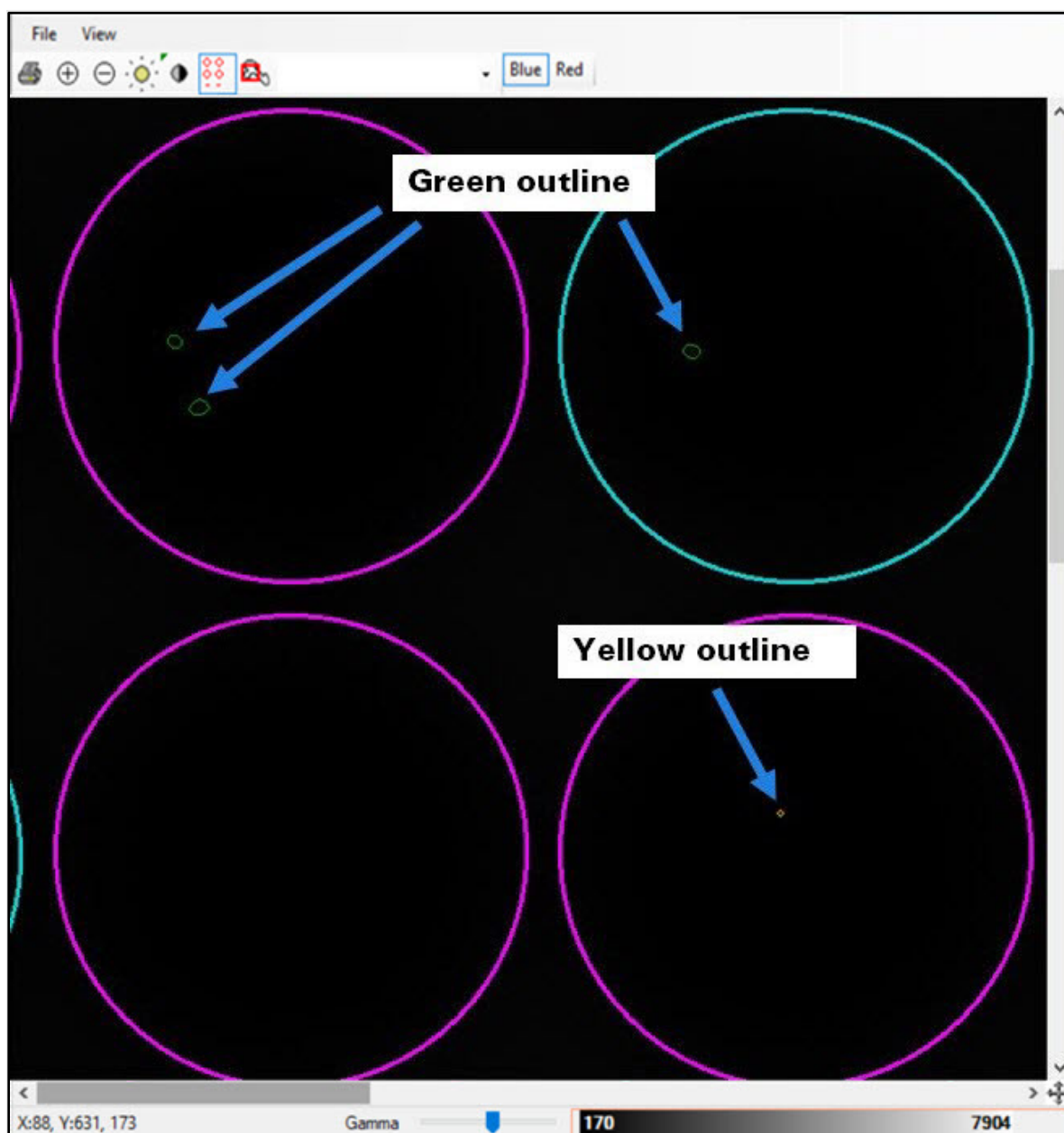
Figure 43. Closeup of wells, showing cell outlines. Green outlines are highlighted in the top wells, while a yellow outline is exemplified in the well on the bottom right.
