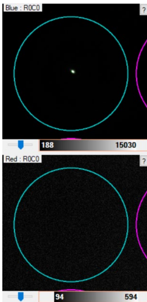
Figure 46. Single-well image from a two-color chip scan of cells stained with Hoechst (Blue channel) and propidium iodide (Red channel). The top image shows cells that have absorbed Hoechst, which indicates the presence of one or more live cells. The bottom image would show cells that have absorbed the propidium iodide, which occurs if a cell is dead; a live cell is not expected to absorb propidium iodide and, therefore, should not appear in the bottom image. In this example, the well matches the designated candidate logic selection parameters (see Section II.C ) and is, therefore, a candidate. If objects appear in the bottom image only or both the top and bottom images, they are either dead cells or an imaging artifact.
