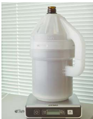
Figure 2. Pressure reservoir on the electronic scale
