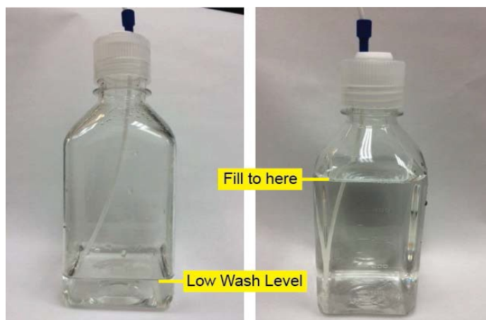
Figure 9. The wash bottle, illustrating a low level and the fill line
