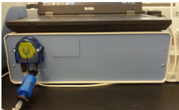
Figure 5. Front view of the peristaltic pump control box and environmental controller
