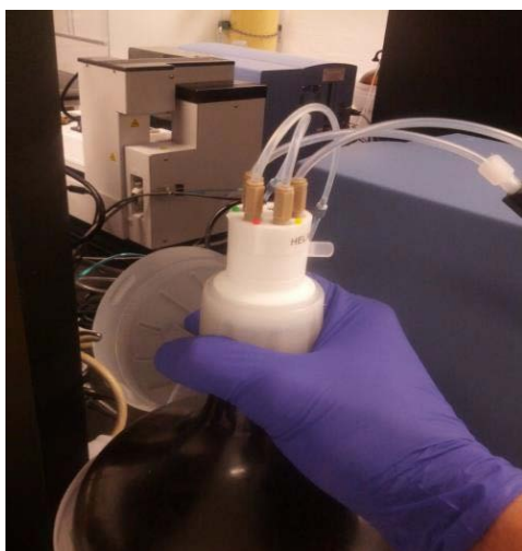
Figure 33. Removing the pressure reservoir cap unit.
