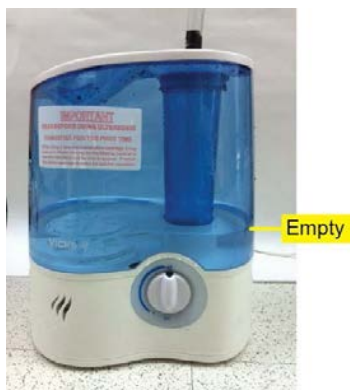
Figure 10. The humidifier reservoir and the level at which the reservoir should be refilled
