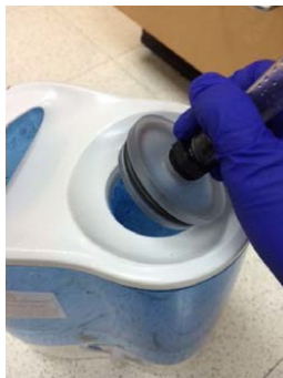
Figure 15. Hose adapter unplugged from the top of the humidifier
