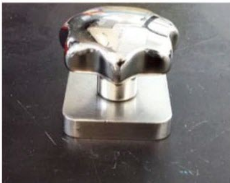
Figure 12. Blot the chip with blotting paper and a blotter. A blotter is provided with the ICELL8 Single-Cell System (Cat. No. 640000).
