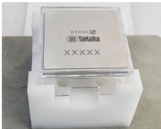
Figure 42. Placing the chip into the Collection Module.
