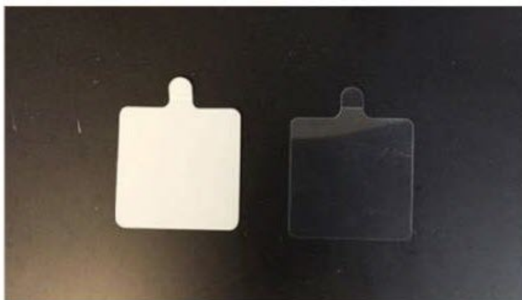
Figure 13. Sealing film and imaging film. The sealing film (left) is provided with a white backing. The imaging film (right) has three layers; the intermediate layer is double sided and is provided between two layers of clear backing.
