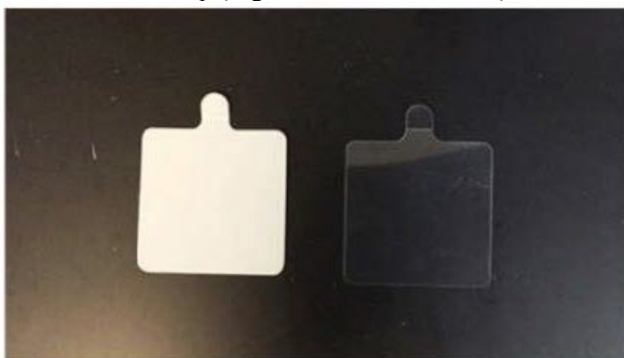
Figure 14. Sealing film and imaging film. The sealing film (left) is provided with a white backing. The imaging film (right) is double sided and is provided between two layers of clear backing.
