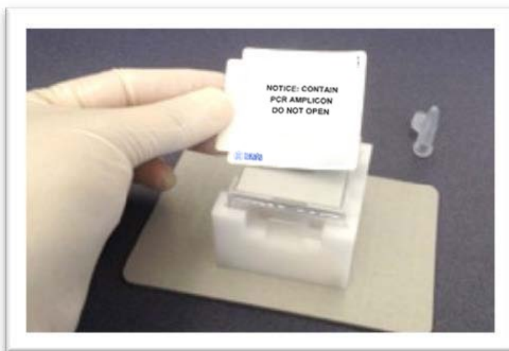
Figure 45. Securing the Collection Module with Collection Film.
