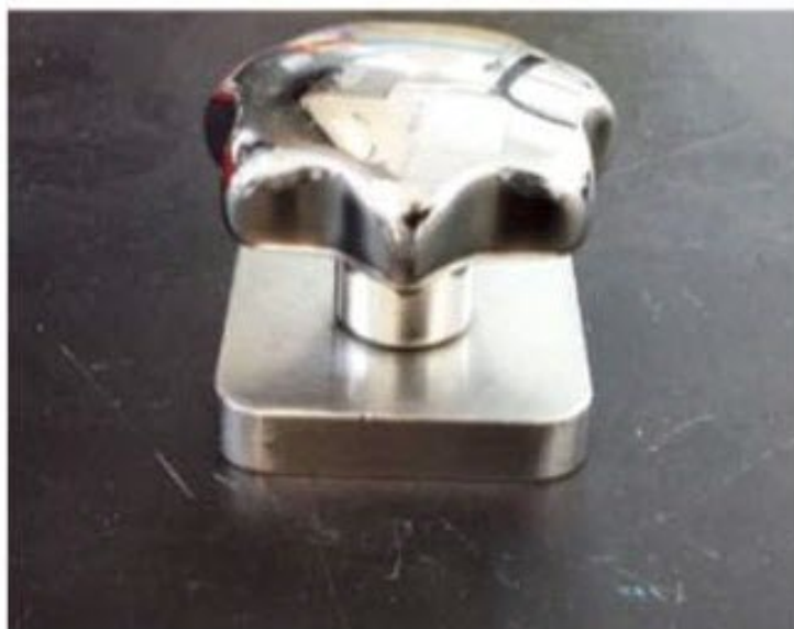
Figure 13. Blot the chip with blotting paper and blotter.
