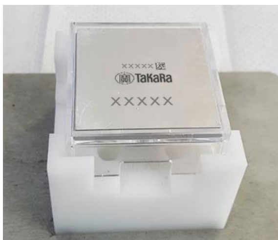
Figure 44. Placing the chip into the Collection Module.
