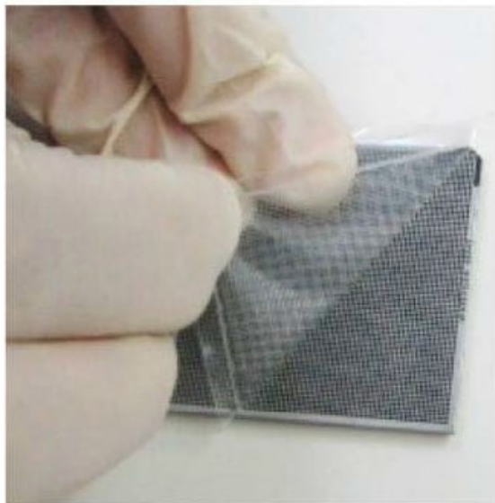
Figure 43. Removing the PCR sealing film from the chip. Start from one corner and apply even pressure to pull.
