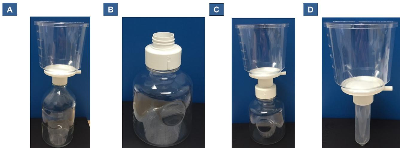
**Figure 1. Setting up the Capturem His-Tagged Purification Large Volume Unit.** The Capturem His-Tagged Purification Large Volume Unit connects directly to a 33-mm diameter thread bottle (**Panel A**). The provided Bottle Thread Adaptor (**Panel B**) allows the purification unit to connect to a 45-mm diameter thread bottle (**Panel C**). The purification unit connects directly to a 50-ml tube for elution (**Panel D**).
