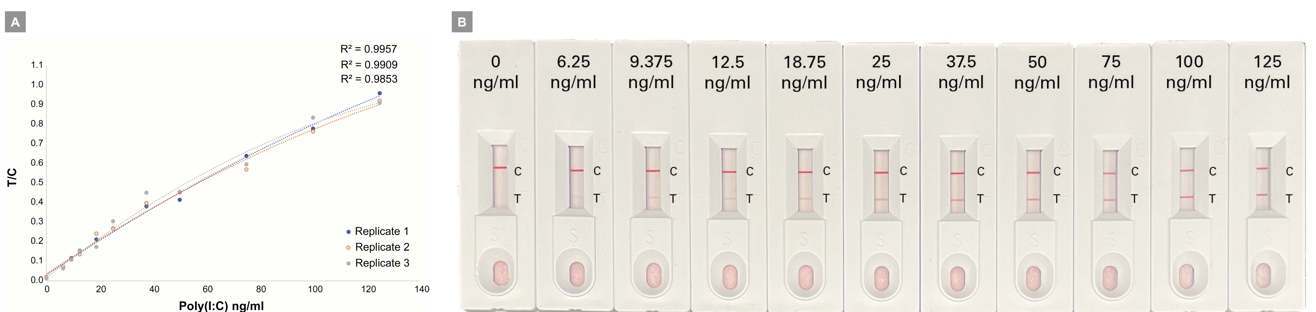
Figure 5. Establishment of control curve. A standard curve was generated using average T/C values from a dilution series of poly(I:C) prepared in chase buffer (Panel A). Samples were run on GoStix Plus cassettes in triplicate, developed for 10 min (Panel B), and analyzed using the GoStix Plus App on both iOS and Android devices. T/C ratios corresponding to each poly(I:C) concentration were plotted to create the standard curve (Panel A). This standard curve is preloaded in the app and does not need to be recreated by the user. When poly(I:C) is used as a reference, the app uses a linearized equation from this curve to automatically quantify dsRNA levels in unknown mRNA samples, with results reported in ng/ml of poly(I:C) equivalents.
