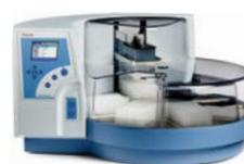
Subsequent DNA isolation is performed on the automation platform KingFisher<sup>®</sup> Flex. The isolation principle is based on reversible adsorption of nucleic acids to paramagnetic NucleoMag<sup>®</sup> B-Beads under appropriate buffer conditions.
