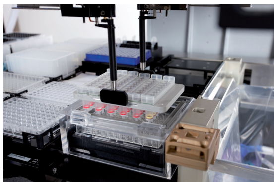
Figure 1: Transport of 8-well strips placed on the adapter plate to the CVS vacuum station using the Hamilton CO-RE Gripper. In the background, the HAMILTON Heater Shaker can be seen.
