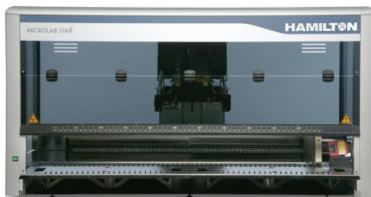
Figure 1: A MICROLAB® STAR, equipped with 8 individual 1000µl channels was used in this study.
