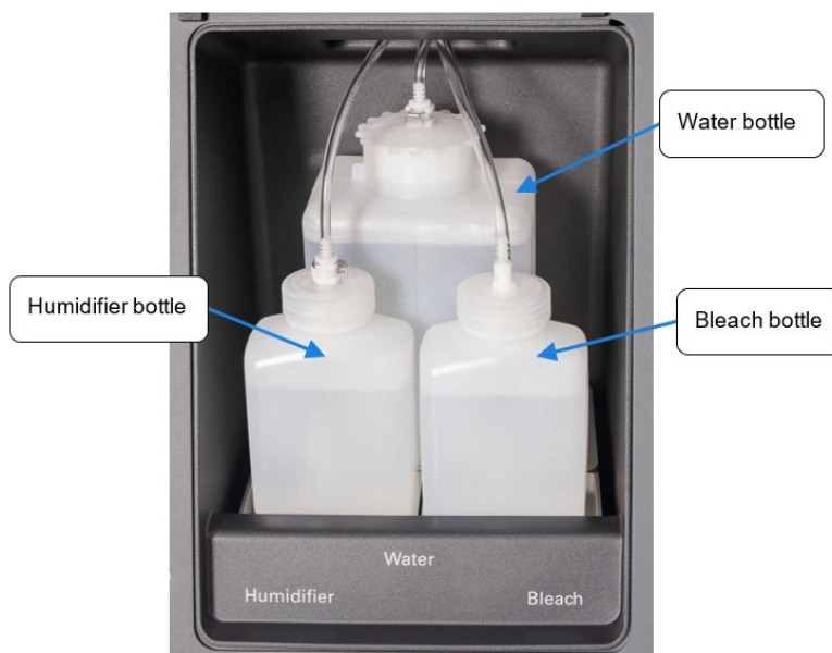
Figure 8. The Shasta Single Cell (internal view), source bottle positions.
