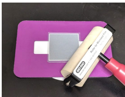
Figure 67. Sealing the chip with film and a film-sealing roller. The chip is being sealed while placed in the Nanodispenser Chip Centrifuge Spinner.
