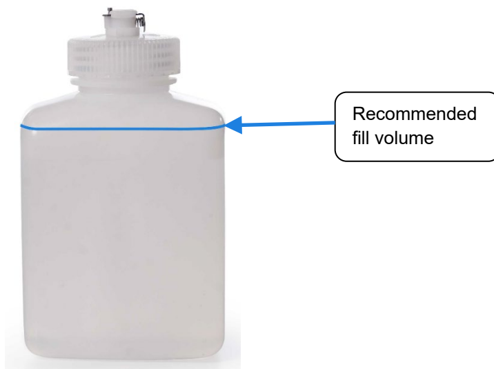
Figure 81. Visualization of the recommended fill volume of the humidifier source bottle. The water level should be below where the bottle begins to curve to the top.
